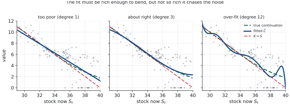
Figure 8: Choosing the regression basis. Left: a straight line cannot bend to the curvature of the continuation value (green dashed truth). Centre: a degree-3 polynomial tracks it well. Right: a degree-12 polynomial over-fits, wriggling to chase noise—harmless in the dense middle, dangerous at the sparse edges where it can mis-rank paths against the exercise line. Rich enough to bend, not so rich it chases noise.
